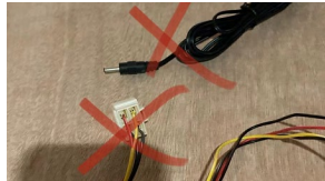
Figure A-7: No connection of wires
